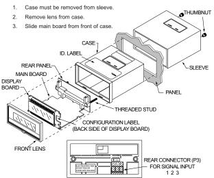
Figure 3-1 Exploded View (includes rear panel)
